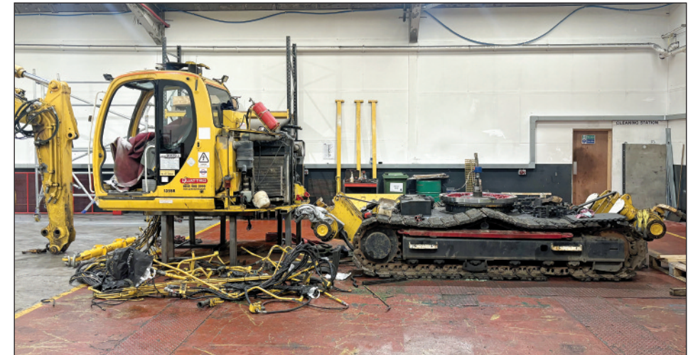
Below: A road/rail 360° crawler excavator stripped down in the process of receiving a RIS-1530-PLT Issue 7 upgrade.
